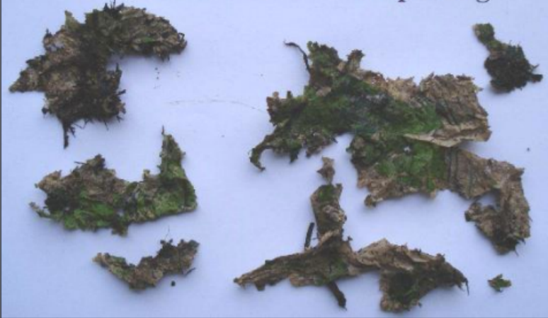
EN 13432 certified biodegradable plastic bag Bio 2 (30 µm) After 2 weeks of composting
