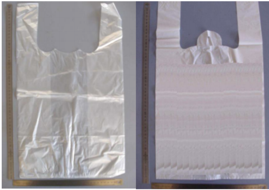
EN 13432 certified biodegradable plastic bag Bio 2 (30 µm) After 2 weeks of composting
